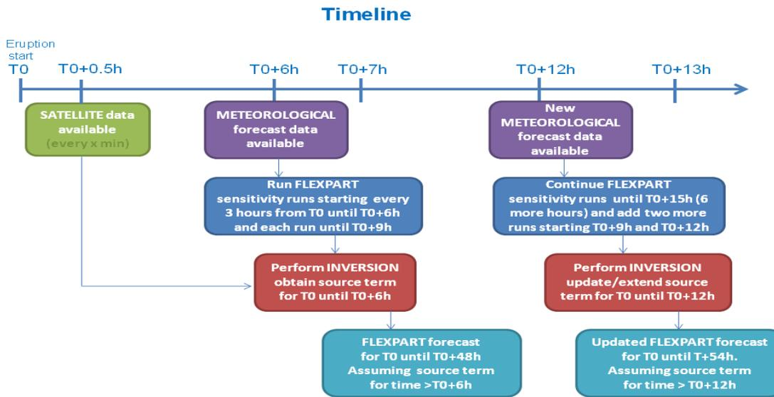
Figure2: Diagram of the updates in the source term estimates as new GFS meteorological incoming data is available to the system, with, in this case, two source term estimates per day.
